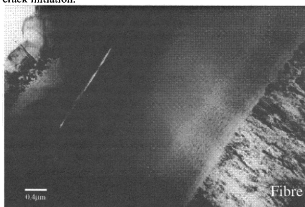
Figure 12 Textron SCS-6 Fibre Coating
