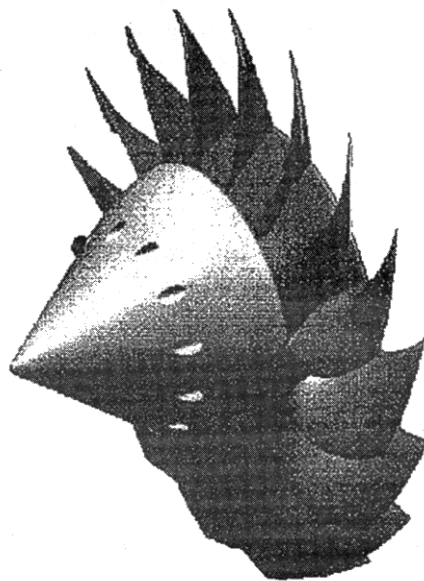
Figure 13: CAD Solid Model of the Compressor Rotor Assembly
